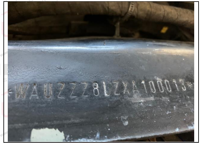
PHOTO Chassis Identification Number
