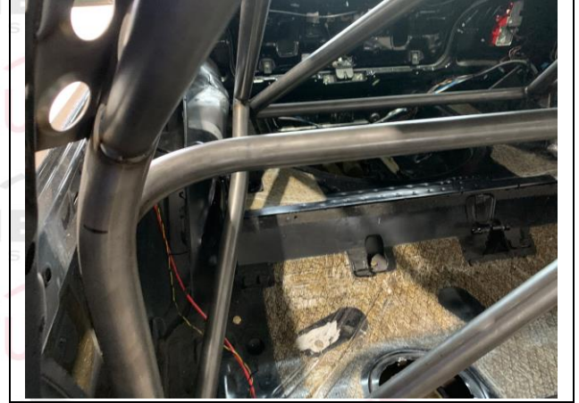
PHOTO 13 SHOULDER HARNESS ATTACHMENT - CO DRIVER
