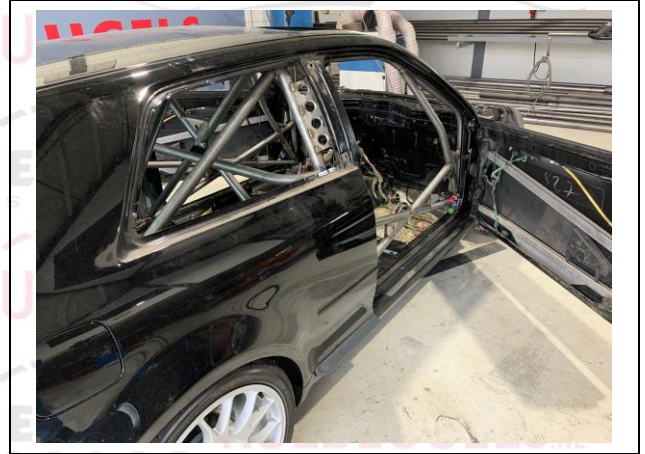
PHOTO 2 REAR ¾ VIEW OF CAGE
